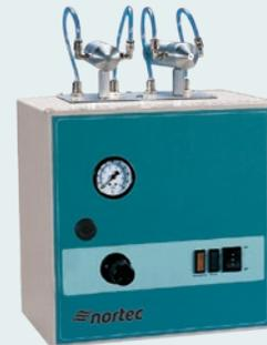
The unique **STAGE VALVE ASSEMBLY** allows you to obtain up to six stages of output through the nozzles. The valve **CONTROLLER** receives a control signal from the building management system will activate combinations of valves to modulate the humidity output.
